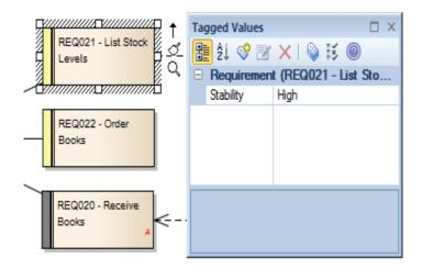
Figure 6: Requirements Tagged Value dialog allowing the assignment of Attributes
