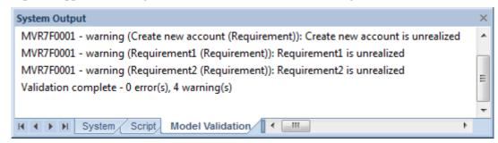
Figure 17: Using Model Validation to check for unrealized requirements
