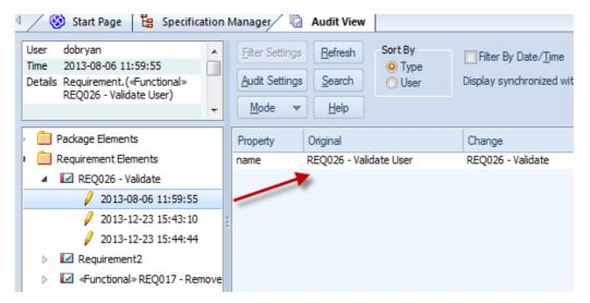
Figure 18: Audit view showing a list of alterations with the details of a Name change shown
